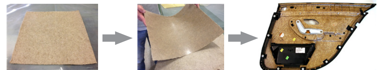
Flax nonwoven impregnated with acrylic resin
